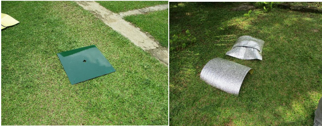
Photo 1 and 2: PVC ceiling sheet and insulation shield that was used to control the heat in the roof
